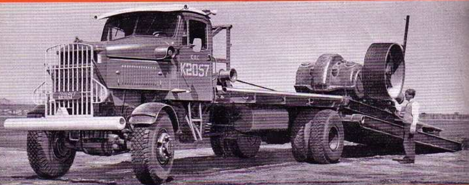
"Mountaineer" 19' Wheelbase Oilfields Truck with a load capacity of 22,000 lbs. showing winch being used to load unitized equipment.
