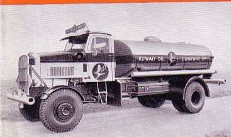
"Mountaineer" 17' Wheelbase Tanker. Capacity 2,500 gallons. Discharge by power driven pump through flowmeter.
