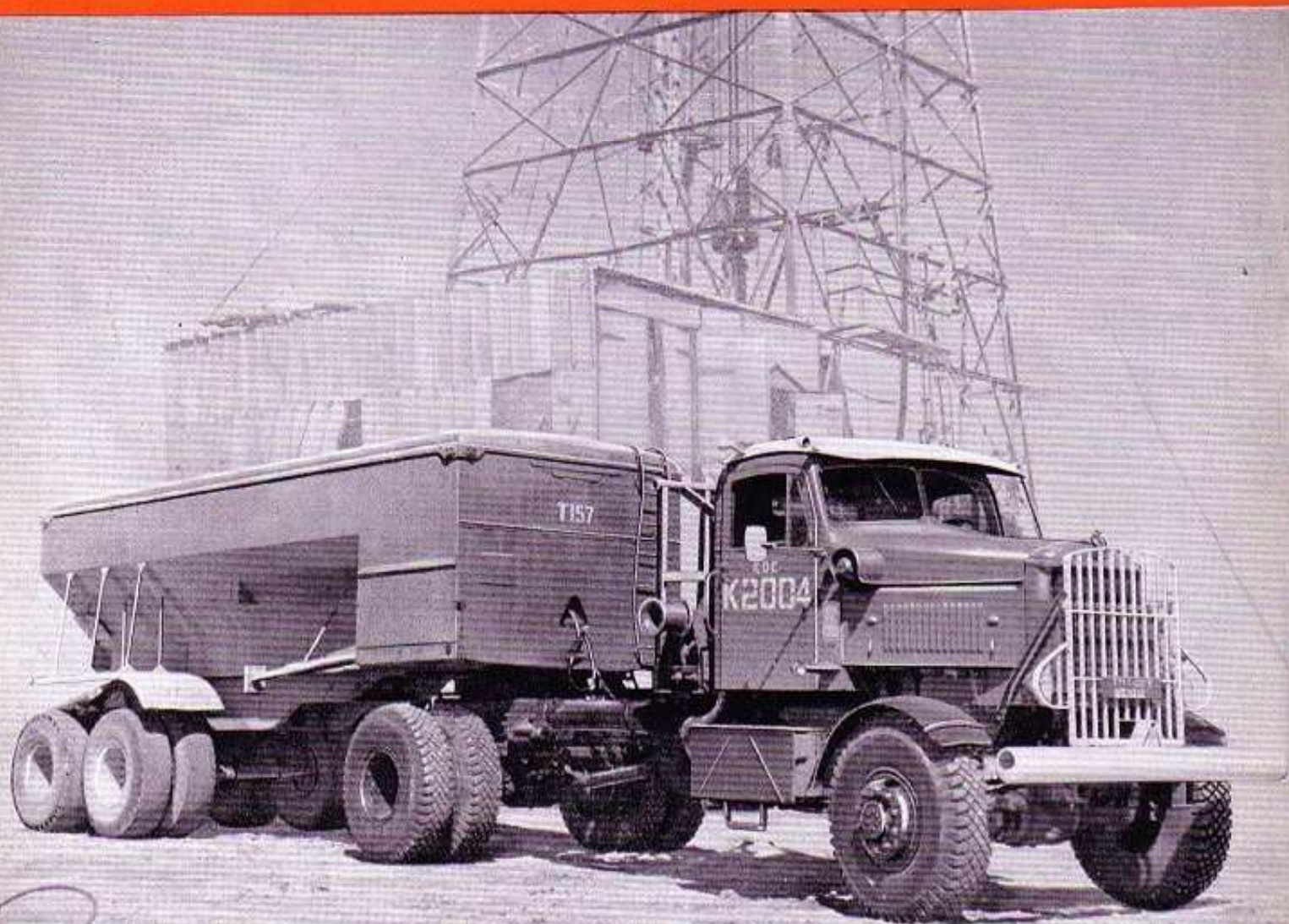
"Mountaineer" 19' Wheelbase Oilfields Truck with a load capacity of 22,000 lbs. showing winch being used to load unitized equipment.
