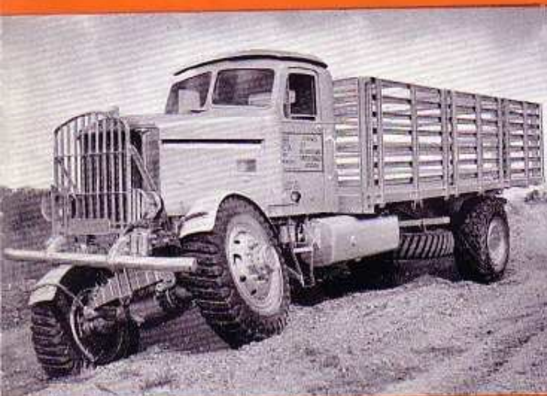
"Mountaineer" 19' Wheelbase "off the highway" Truck. One of a number operating over virgin territory for carriage of locust balm in Saudi Arabia. 130 h.p. engine provides ample power for trailer towing if necessary.
