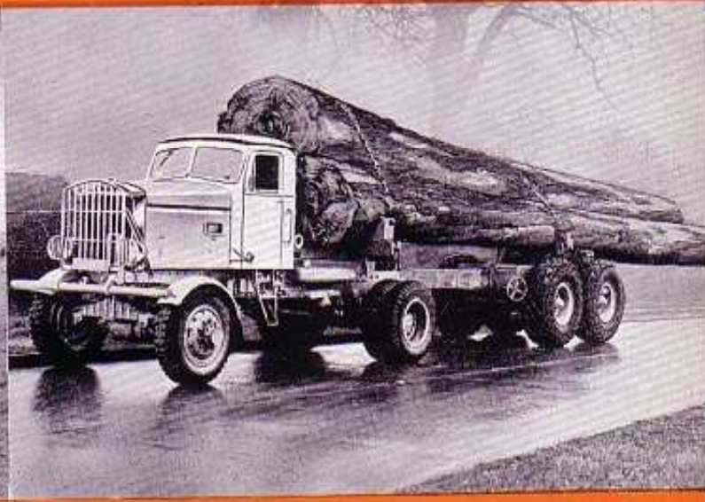
"Mountaineer" Articulated Timber Transporter 14' Wheelbase Motive Unit with 25 ton extensible Pole Trailer for forestry operation.
