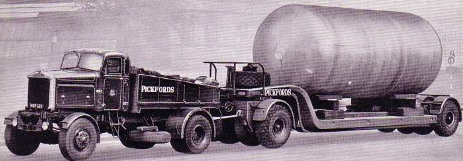
"Mountaineer" 14' Wheelbase Tractor with drawbar trailer for abnormal indivisible loads. Suitable for gross train weights up to 134,400 lbs.
