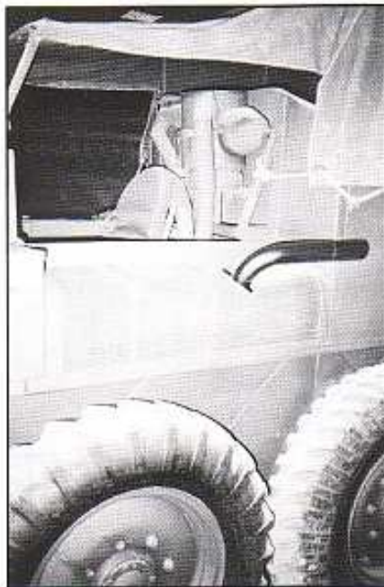
Above: Prototype No. 1 under test. Notice the neat finish of the body panels. Approximate dims. in metres: overall L×W×H 3.50×1.35×2.30; wheelbase 1.10+1.10; track 1.15.
