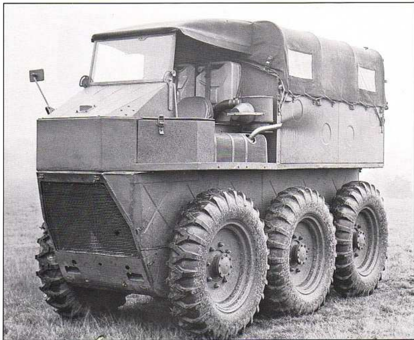
This and the following three are probably the sole official works photographs of the Hexonaut in existence today. Humber Ltd's Engineering Department captioned them: '15-cwt 6x6 GS Vehicle; designed to be carried in Dakota aircraft; prototype No. 1.'
