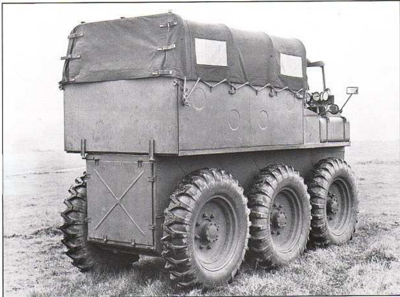
Among detail differences between No. 1 and survivor (shown) are air cleaner set-up and location of radiator filler cap. Access to cab and power train are extremely poor.
