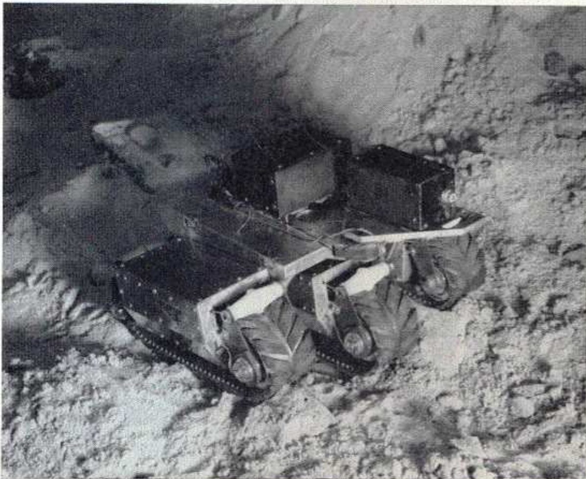
FIG. 14. Simple yet compact 3 \times 3 ELMS stowage concept. For deployment front unit drives forward under its own power.
