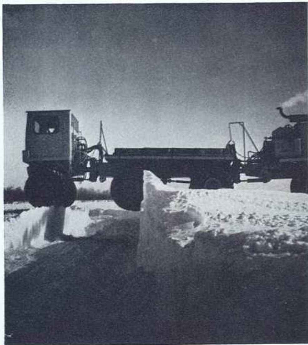
FIG. 4. Trench bridging, 8 ft wide.
