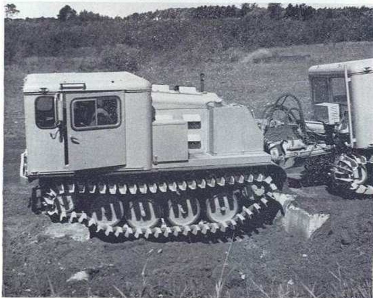
FIG. 6. Trench bridging 10 ft wide.
