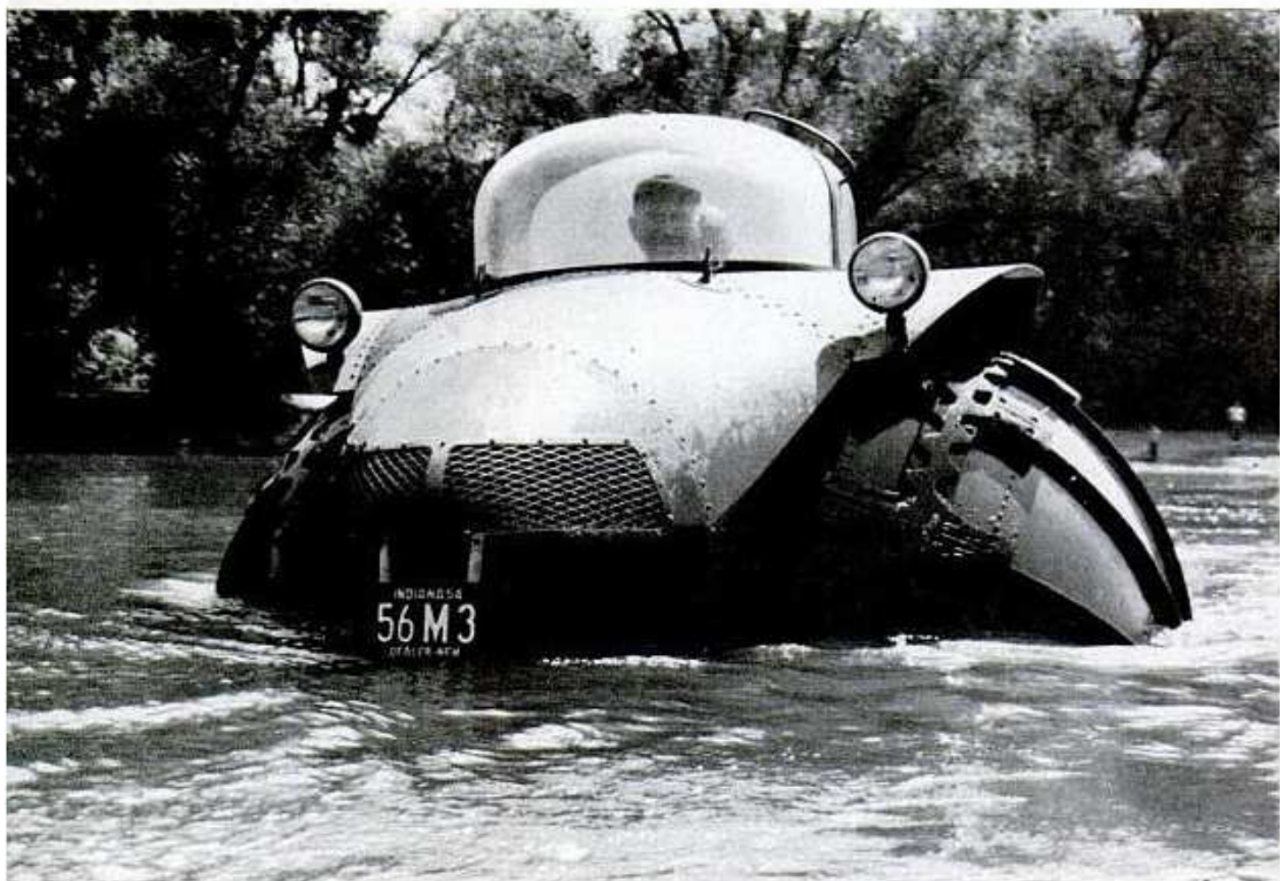
HOLLOW WHEELS and seam-welded body keep Rhino afloat. It makes five m.p.h. in water, up
