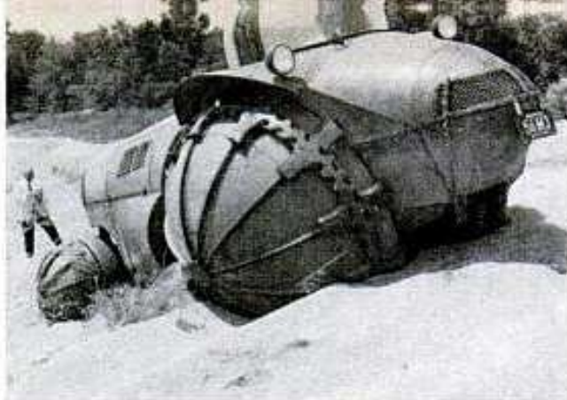
ON FOUR-WHEEL DRIVE the Rhino claws through sand, climbs 65-percent grades. Aluminum front wheels, twice as big as the rear, are six feet in diameter and weigh 1,500 pounds each.
