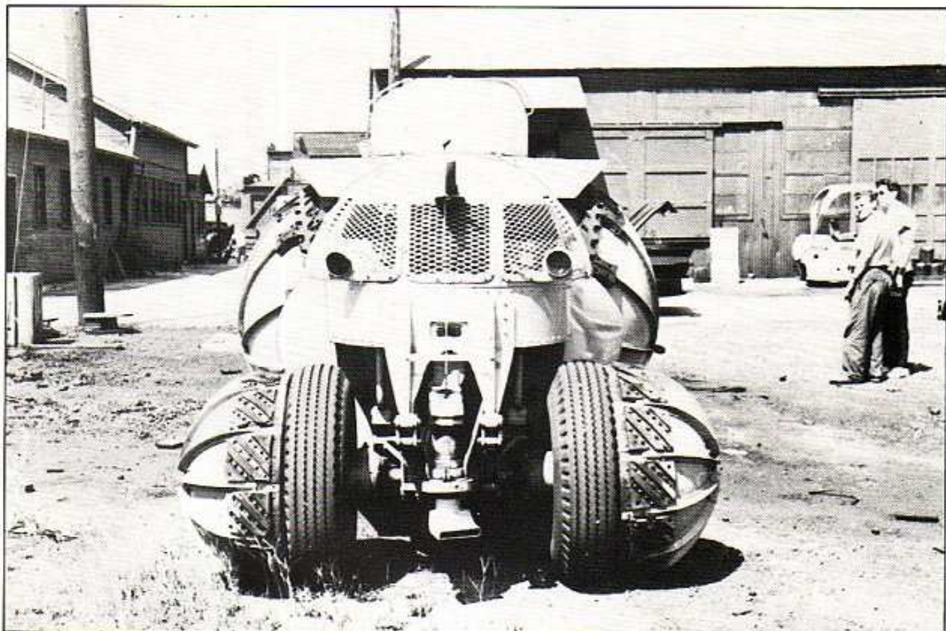
The 'Rhino' in Marmon-Herrington factory yard in the late 1950s. Note the swivelling hydrojet unit between the (rear) wheels.
