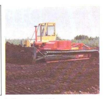
The DIFCO BOGMISER can operate a wide range of Ditching Equipment on its 3 pt. linkage.
