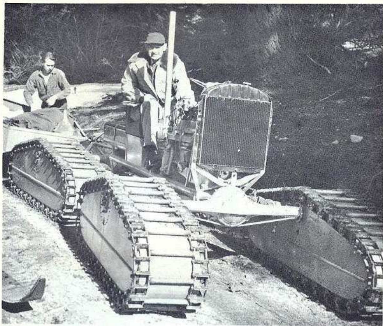
Fig. 14. Prototype Tucker SNO-CAT, about 1948
