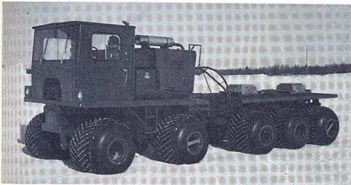
FIG. 21. VEXA 2½ ton 10×10 Mobility Test Rig. (U.S. Army photograph.)
