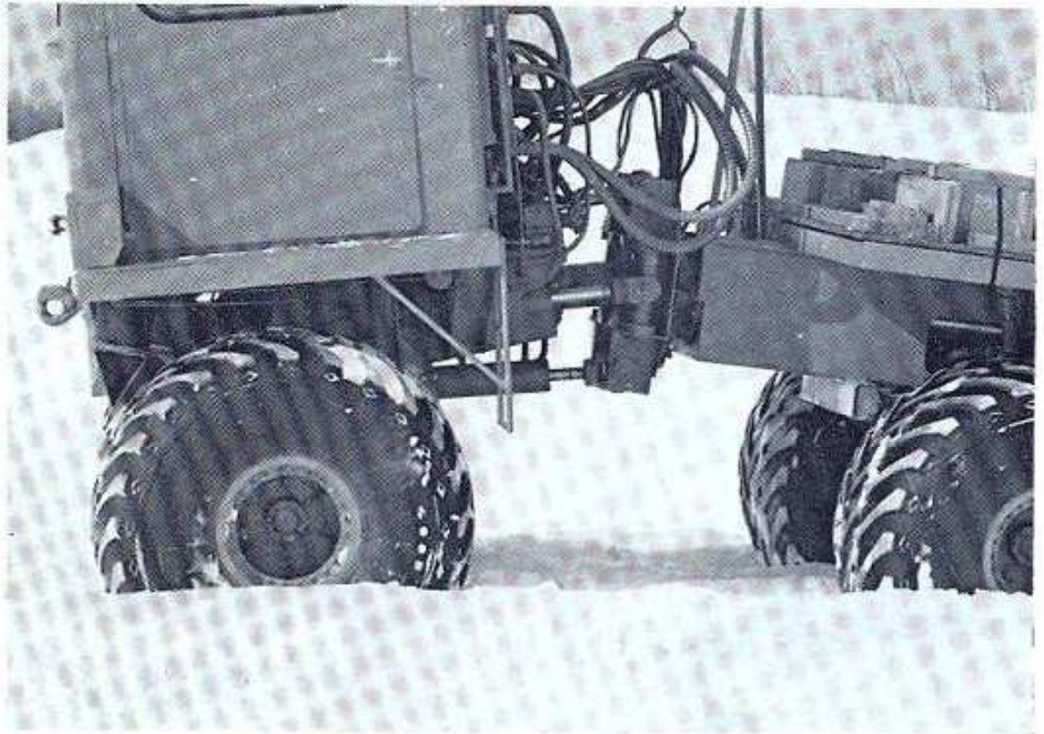
FIG. 27. The VEXA vehicle joint with active pitch control and inching system. (U.S. Army photograph.)
