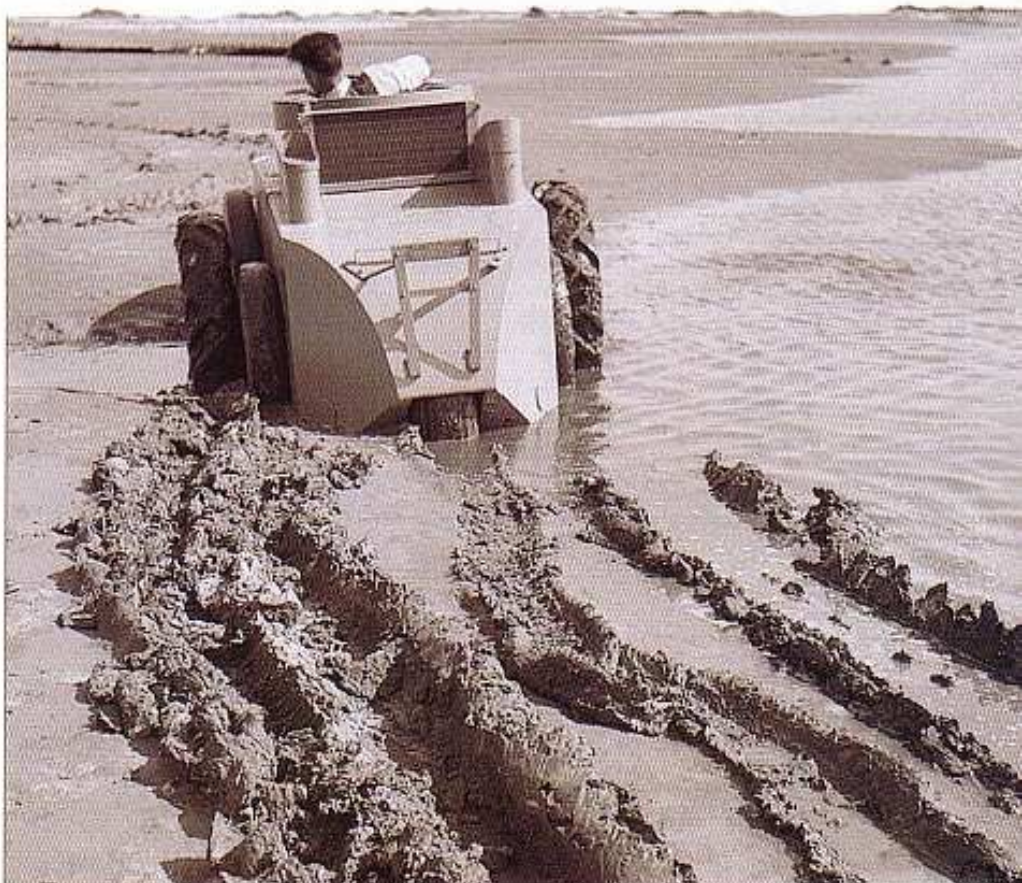
Ooo...er... in wet sand, the multiple wheelbases of the Scorpion leave a very distinctive trail. (IWM, H19428)
