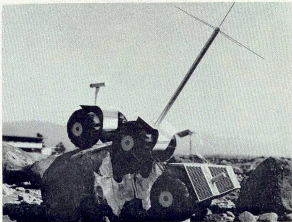
FIG. 3. A small remote control lunar rover equipped with elastic frame negotiates an obstacle.
