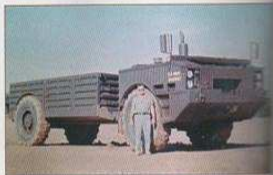
The side panels of the cab portion of production vehicles were corrugated for added strength. The front winch, missing from this vehicle, was a standard Ordnance model, and was recessed into the front panel. In most applications this winch is powered via a power take-off shaft, but when installed on the Goer, it was driven by a hydraulic motor. (Courtesy, History Office, US Army Tank Automotive Command)
