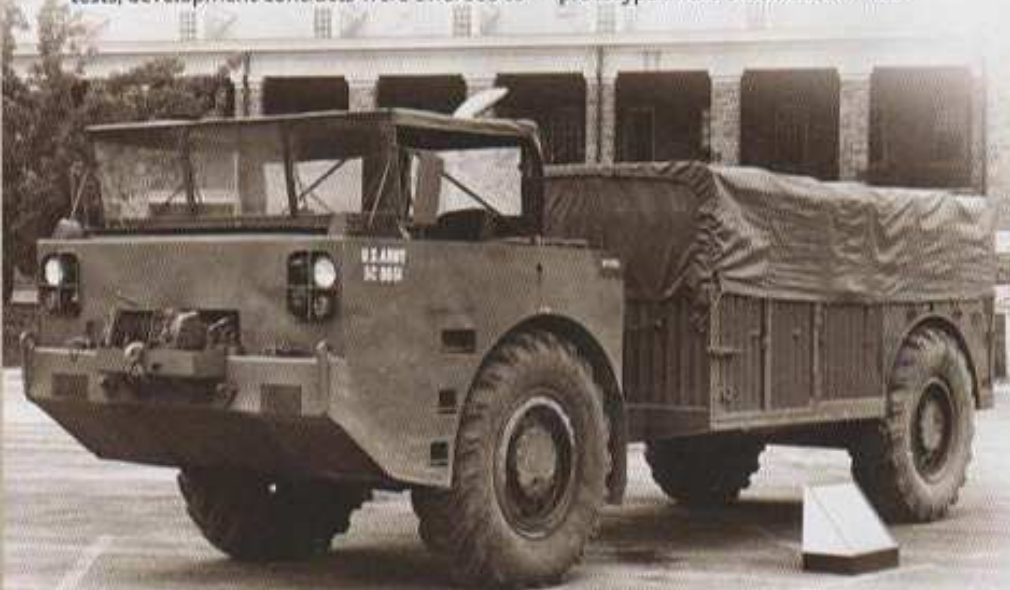
Further developments resulted in this 1965 version of the XMS20E1. It used the same engine as its predecessor, but this was now coupled to a six-speed transmission with torque converter and planetary drive. The cab was redesigned, reducing the vehicle's overall length. The self-recovery winch installation was also revamped completely. (Courtesy, Patton Museum, Fort Knox, Kentucky)
