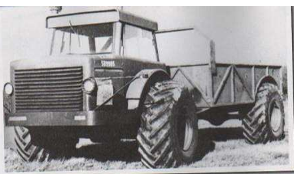
The earliest member of the Goer family was this vehicle built by Clark Equipment Company. Based on their Michigan Division Model 75 log skidder. Clark's machine was powered by a Cummins six-cylinder diesel engine. (Courtesy, Patton Museum, Fort Knox, Kentucky)
