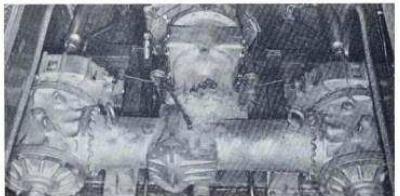
Differential transmission details
