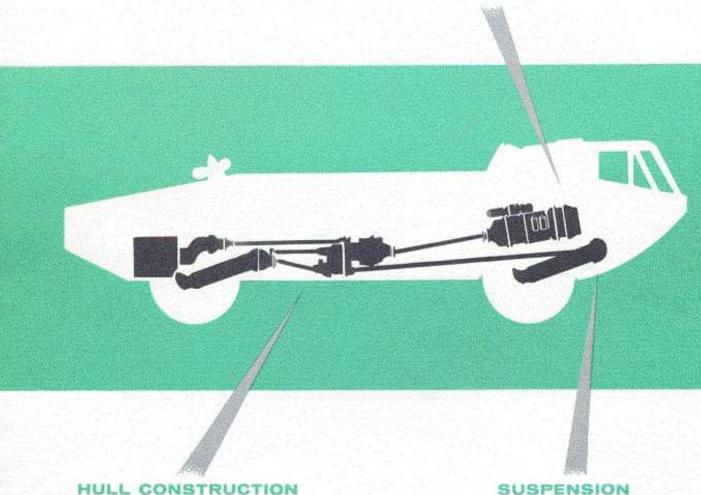
The hull of the LVH combines optimum weight and strength characteristics for all operational conditions. It is an integrally stiffened box structure of aluminum and stressed skin in accordance with conservative aircraft design practice. Overall dimensions were designed to allow operations from the LST, LPD and LSD.
