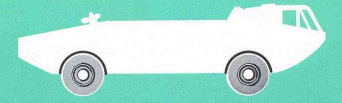
With wheels extended for normal overland operation the cargo bed is five feet above ground level. The oleo strut suspension system makes possible a smooth ride at all road speeds and reduces stress levels in the hull during land operation. Only 12 seconds are required for either extension or retraction of the wheels. In addition, wheels may be individually retracted for ease of maintenance.
