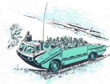
The easily accessible cargo compartment of the LVH has a capacity for transporting five tons of cargo of all types, or large numbers of fully equipped personnel. The compartment sides fold down to become loading ramps, eliminating the need for large cranes or other specialized material handling equipment for normal loads. These ramps are of high-strength honeycomb construction to withstand the characteristic abuse of cargo handling.
