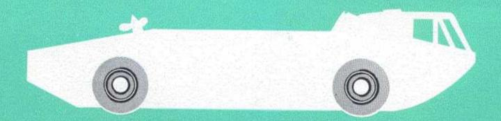
The LVH design incorporates a unique wheel retraction and an independent wheel suspension system in a single unit. This system is capable of lowering or raising the amphibian with its maximum payload of 10,000 pounds. By retracting the wheels, loading or unloading of the vehicle is readily accomplished without the use of specialized handling equipment.
