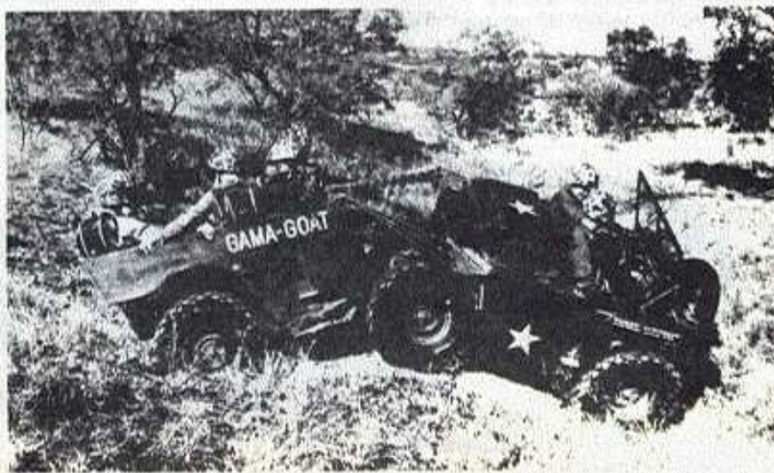
Fig. 4—"Gama Goat" prototype of XM561 six-wheeled articulated truck now being developed for the U.S. Army
