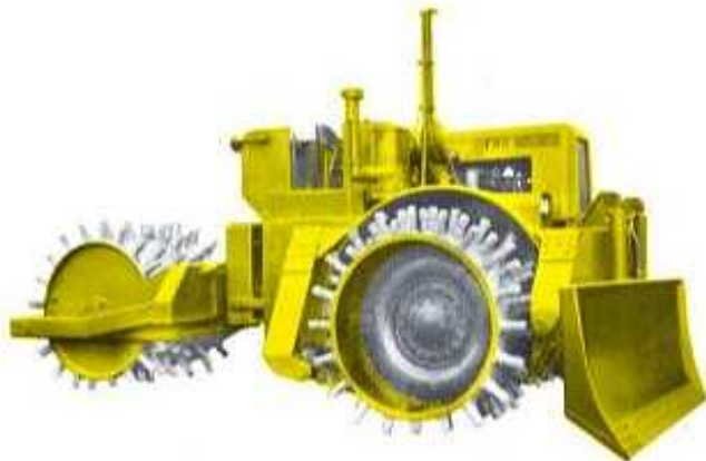
WC-24 Sheepsfoot Compactor built for Bureau of Reclamation work, dams, levees, etc.
