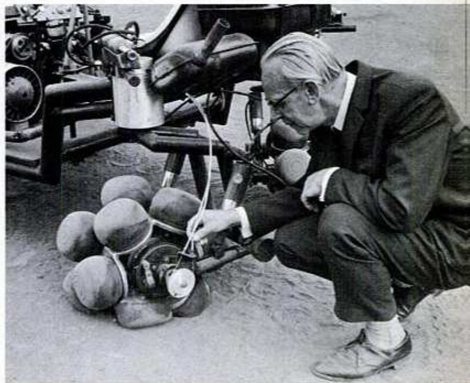
The inventor of the Rotoped — Julius Mackerle — checks on a cable connection to a wheel hub. When the vehicle is at a standstill, the bags in contact with the ground are partially deflated.
