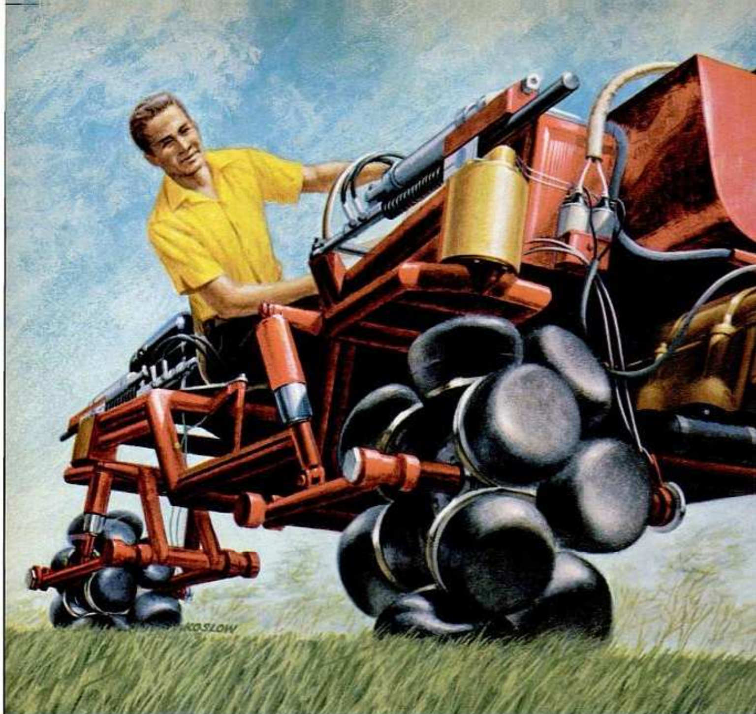
Trabant engine in nose of the Rotoped drives a blower that feeds compressed air via tubular
