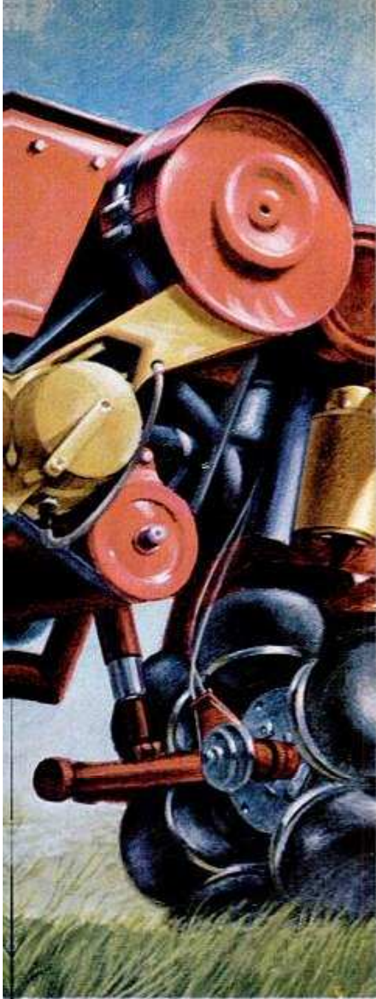
All driving machinery is crammed into the front of the chassis. The controls are no more complicated than those in a modern car, but the Rotoped's off-road mobility may be unequalled.
