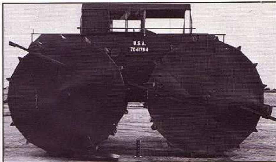
The Higgins-built amphibian at Aberdeen Proving Ground seen here with and without its 40-inch 'steppers'. Reportedly (and not surprisingly) it was also tried with steel rings welded around the wheel outer edges to improve the ride on hard ground. Stencilled below the USA registration number was 'Swamp Skipper 327-22-000' (hardly visible here). The Automotive Division Test number was 764.
