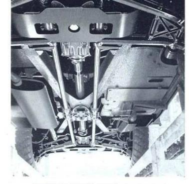
A general underneath view showing the sturdy semi-integral construction of the body.
