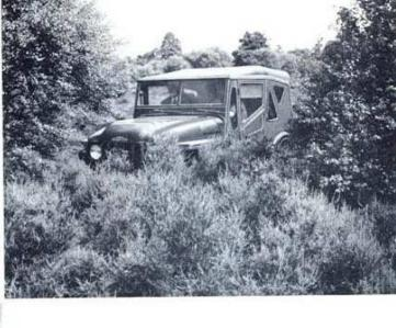
The "Champ" is fitted with a towing attachment as standard equipment and provision is made for fitting a power take-off unit or winch. Thus, in addition to its numerous other applications it may also be employed in recovery work, driving machinery and hauling.
