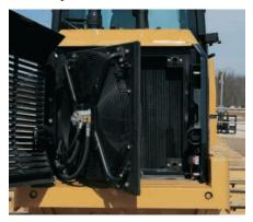
**Cooling System.** The fan and the grill swing open, providing excellent access for clean-out and maintenance. The heavy duty latched grill minimizes debris build-up.
