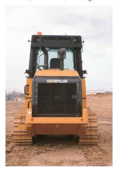
**Rear Engine Location.** Rear engine location allows excellent forward visibility, while serving as a working counterweight. It also helps reduce radiator plugging while providing easy service access to the engine and other major components.
