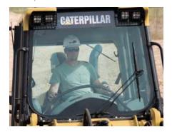
**Viewing Area.** Large windows use tinted glass to reduce glare and provide an excellent view to the bucket, tracks, and around the engine enclosure to the rear.
