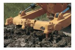
**Ripper-Scarifier.** A radial ripper-scarifier is available for the 963D as an attachment. It is mounted with two pins pressed into each side of the main frame. Two cylinders raise and lower the ripper. The ripper beam has three pockets for holding ripper shanks. The linkage pins do not require lubrication.
