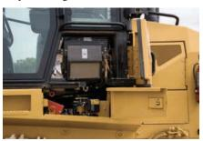
**Cab Air Filter.** The cab air filter, the grouped pressure taps, the cab tilt locking bar, the optional cab tilt cylinder, the tool box, and the hydraulic oil filters are conveniently located below the left-side cab window.
