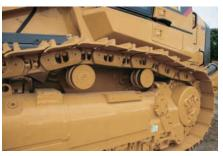
**Carrier Rollers.** The 963D has seven track rollers, which spread machine weight over a large area and two upper carrier rollers on each side mounts to the machine mainframe.
