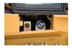
**Fuel fill.** The fuel tank and the optional quick fill port are located on the right side compartment, below the cab access.
