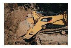
General Purpose Bucket. The General Purpose (GP) bucket is designed for excellent loadability and long life in a broad range of applications such as hard bank excavating, stripping and stockpile loading. High-strength, low-alloy steel helps the bucket resist dents and abrasions. Rear edge of bucket is designed for improved efficiency when backdragging.
