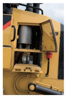
**Left side compartments.** The lower part of the compartment door can be used as a step to access the shunt tank fill, the air pre-cleaner (if equipped) and allows easy cleaning of the rear window.
