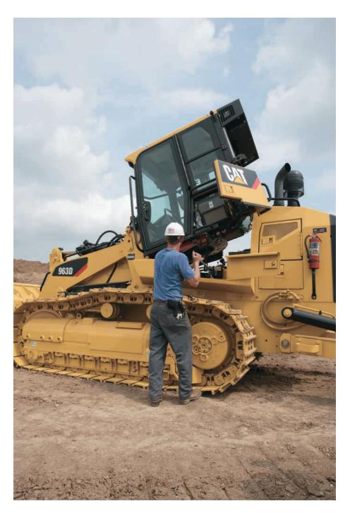
**Tiltable Cab.** The 963D is equipped with a tiltable cab. This new feature makes the maintenance and the repairs easier. By tilting the cab, you can access to the drive train and perform complete service of the hydraulic system.
