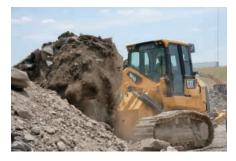
**Automatic kickouts.** The standard programmable automatic kickouts provide flexibility and productivity for precise load and dump target heights. Tilt and lift kickouts are set by positioning the bucket or work tool and setting a rocker switch in the cab.
